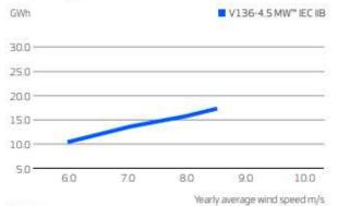
Assumptions One wind turbine, 100% availability, 0% losses, k factor +2 Standard av density =1,225, which speed at hubbleght
