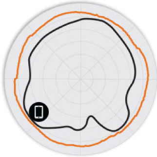
Figure 2. 2.4GHz Azimuth Antenna Patterns
