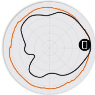
Figure 3. 5GHz Azimuth Antenna Patterns
