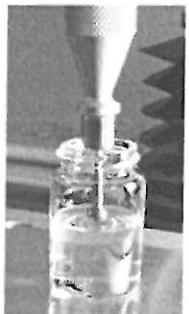
**P/25** **Valcová sonda na meranie lepivosti a elasticity, tvrdosti tablet - 25mm A** **1ks**
